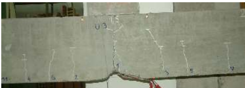
Figure 17. Crack pattern after collapse of beam R50.
