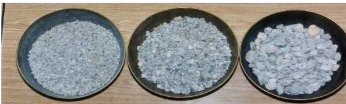
Figure 3. Recycled concrete aggregate fractions. From left to right; 4–8 mm, 8–16 mm and 16–31.5 mm coarse aggregates.
