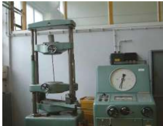
Figure 7. Testing of bond between concrete and reinforcement.
