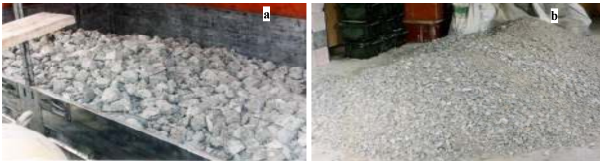
Figure 2. Recycled material after (a) primary and (b) secondary crushing.
